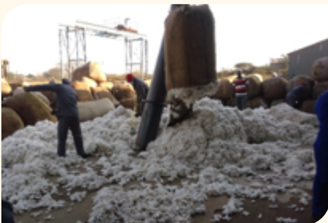
Cotton being offloaded and sucked into the blending rooms
