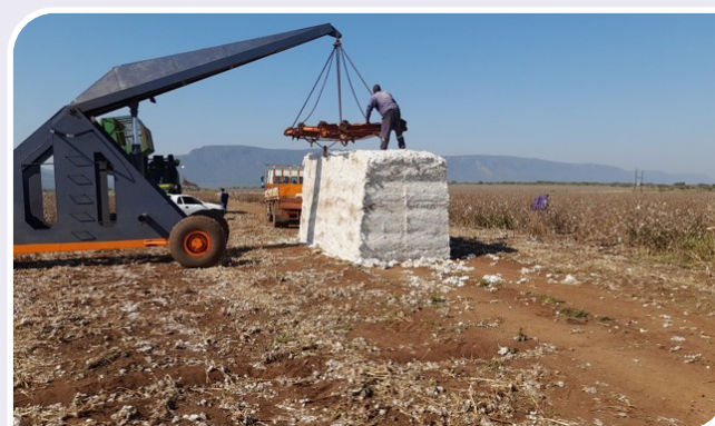
Cotton Module picked up by a crane to deliver at the Ginnery
